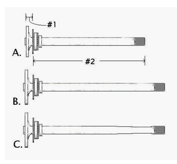
The diagram illustrates 8-3/4" axles. The top is a 66-72 A-body axle. and the other two are longer axles that generally resemble the B and C body and truck axles. C body and truck axles can be shortened and resplined by a quality machine shop, however it is important to note that not all C-body/ Truck axles are created equally.
