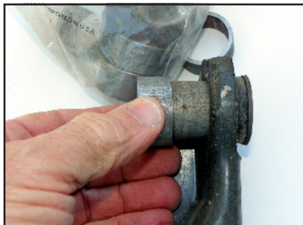
(13) Close-up of aforementioned press collar. Mopar P/N was 1857840. Repros exist. A small mig'd spotweld also works great. Do one or the other.
