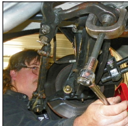
(10) Installation is just nuts and bolts. Step one is to remove the pitman arm. Use a puller, as SSS (SuperStudShaughnessy) is doing here.
