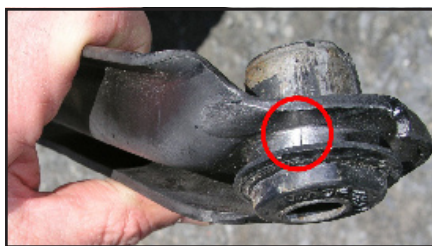
(14) Unfortunately, a bushing swap sometimes causes this type of failure. Weld!
