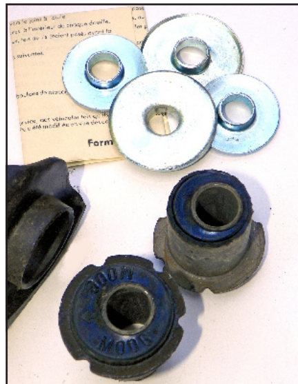
(18) The time-honored fix for insufficient caster has always been offset bushings. Durability is 50-50.
