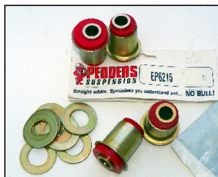
(20) The best of both words can be had—urethane, Pedders P/N EP6215 (a set of 4, enough for two arms). These come from down under, see www.pedders.com.au .
