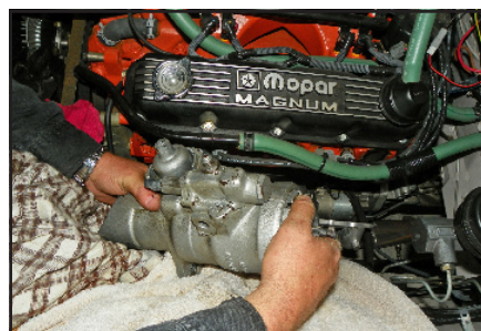
(11) And out it comes. Generally, the left motor mount must be unbolted and the engine jacked, and sometimes the left header or exhaust manifold loosened and swiveled up out of the way. Installation was similarly a cinch.
