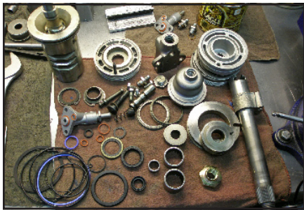
(6) Ready for assembly, with all wear parts either replaced or re-machined to tight tolerances. We went for FFI's "Stage 2" build, which includes beefed reaction springs. Every box is pressure/hot-tested.
