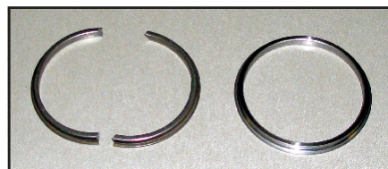
(4) It is very common to find broken reaction spring retainers. FFI replaces these (broken or not) with in-house manufactured high-strength rings.
