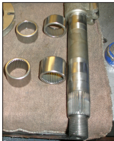
(5) FFI specifies a beefier (wider) lower sector bearing, which further increases precision. On large-spline boxes, the lower bearing can actually be doubled (two installed, "stacked").
