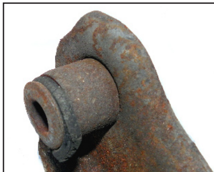
(15) After a few years, stock style rubber bushings aren't pretty. They've gotta go!
