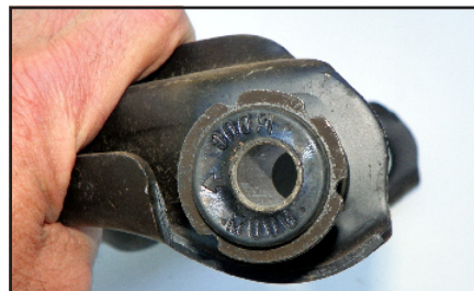
(19) To increase caster, you install the front bushing on each side offset outboard (shown), per instructions, but the rear one with the offset inboard (arrow pointing away from UBJ).
