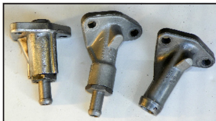
(9) There are myriad return valve bodies, besides differing angles, '67-up used 1 1/2" hose, while '66-down was 3/4". They just bolt on (don't forget the two O-rings). There's also a few pressure fitting versions, all of which can also be swapped. Starting in 1967, the mounting bolts were increased from 3/8" to 1/2", earlier boxes can be drilled for the larger bolts (always make to bolt holes at least 0.040" larger than the bolt, this allows the chuck to wobble a tad to "seat" on the K-member pad).
