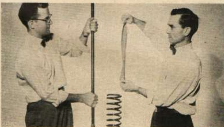
Here is the difference between a straight torsion bar and coil spring. Man on right demonstrates the twist imparted to bar.
