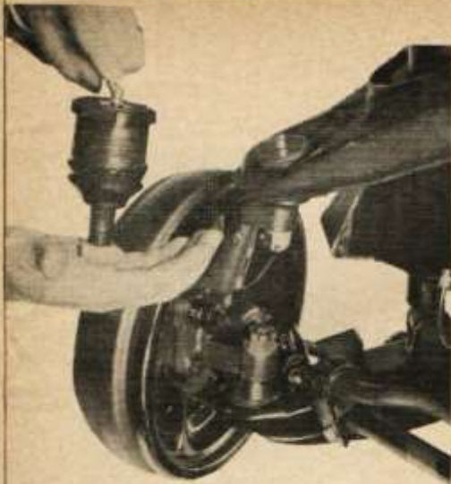
One of the four self-contained ball joints. Lower control arm strut, anti-roll stabilizer mount and snubber also shown.
