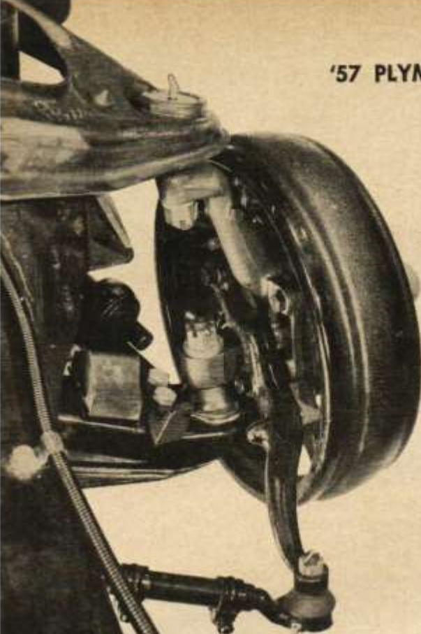
Looking forward from the right side, steering arm and tie rod are shown. Brakes are 11-inch, two-leading shoe type.
