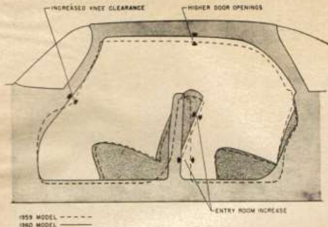
1960 Dodge products have unit construction bodies with larger door openings for easy entry and exit. The floor pan of the cars has also been dropped in 1960 for more comfortable seats.
