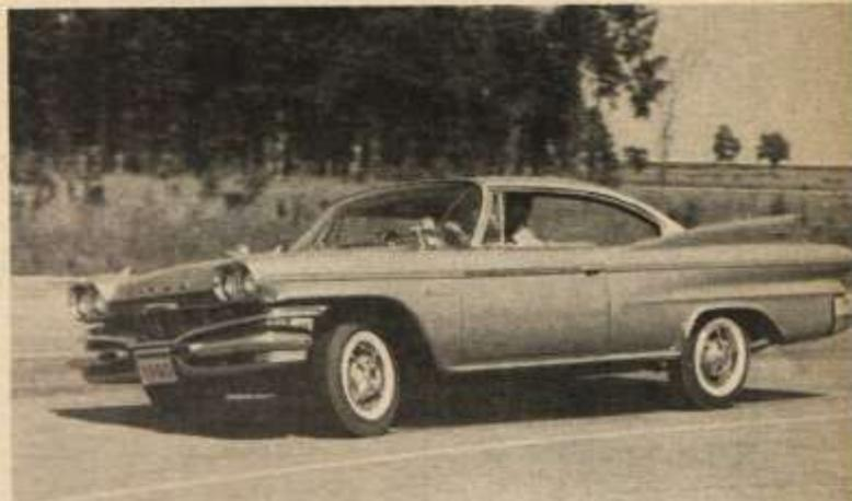
Both right and left turns around circular test pad revealed the 1960 Dodge to have excellent road gripping qualities. Even while leaning to its maximum, Dodge carburetion didn't falter.
