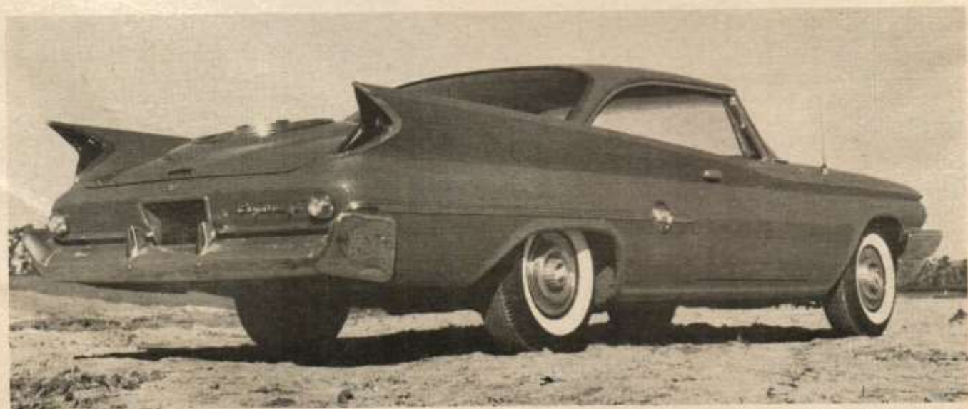
The gasoline filler neck is concealed beneath the rear license plate bracket with a 23-gallon capacity tank. 14-inch wheels are fitted with nylon Supreme grade tires. The 300F Chrysler is available for sale in only four colors; black, white, red and a burnt orange.
