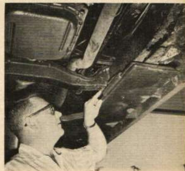
Rear torsion bar adjustment permits raising or lowering front end height of car.
