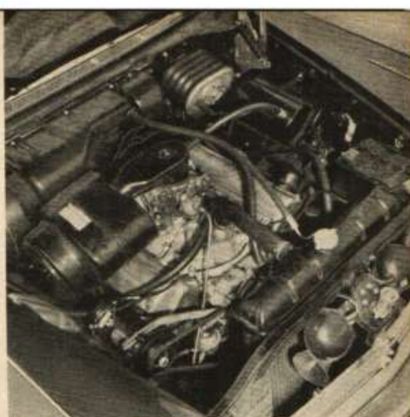
Power pack mill with host of accessories and a single four-barrel carburetor. The V8 ran best with a slight spark advance.
