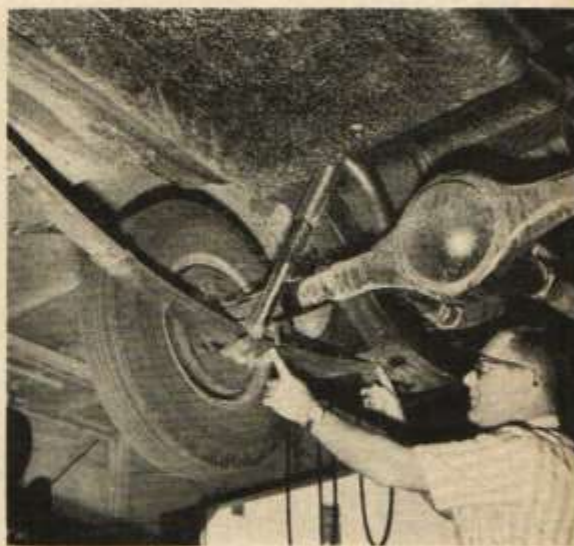
Short forward section of rear spring is a sort of built-in anti-spring-wrap device, absorbing accelerative and brake torques.
