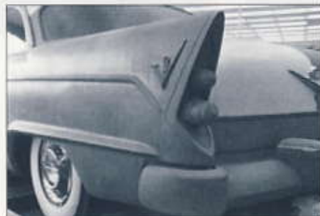
1, 2. Ideas for the 1956 facelift were photographed on June 14, 1954. Note the roof overhang on the driver's side. The rear fin and taillight treatment is surprisingly similar to that of the 1955 Cadillac Eldorado. 3. Ten days later, less-fussy side trim was viewed on the other side of the model. 4, 5. By July 27, the fins and taillamps were getting closer to their eventual form, but the side trim, body sculpturing, and grille were still evolving. The production '56 Dodge would ultimately continue the divided-grille style instituted for 1955.
