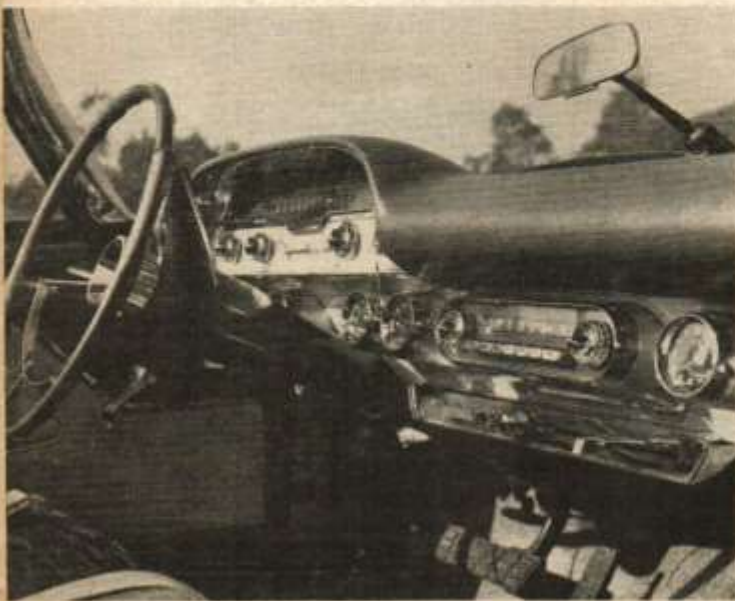
WRAP-OVER WINDSHIELD , available only on the convertible, does not have excessive distortion. However, angle of the glass catches more dirt, makes frequent cleaning necessary.
