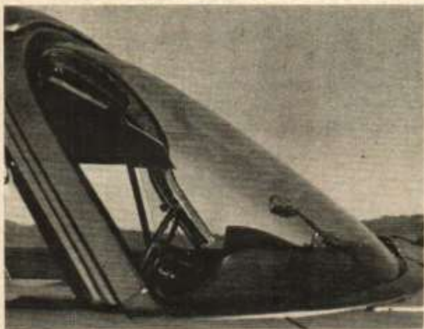
WRAP-OVER WINDSHIELD , available only on the convertible, does not have excessive distortion. However, angle of the glass catches more dirt, makes frequent cleaning necessary.
