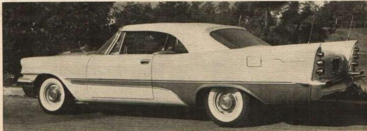
**ENTRANCE AND EXIT** are easy, despite fact that overall height is as low as they come. The reason, common to all 1957 Chrysler Corporation makes, is that the forward post and windshield do not
