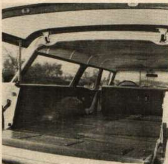
FAST SWITCH from passengers to cargo is simplified on Ford wagon by collapsible seats; nothing has to be removed. Wide rear window opens transom-style.
